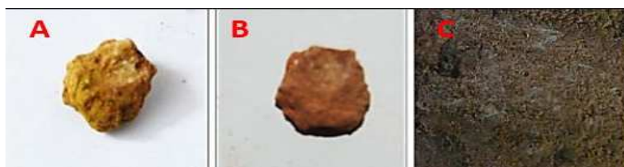
Figure 14. (A) Wall painting before applied Acacia Nilotica , (B) Wall painting after applied Acacia Nilotica , (C) Wall painting after applied Acacia Nilotica using stereo microscope (250x) in faculty of fine arts, Minya University, Photo by the author.
