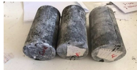
Figure 6. Mode of failure of splitting strength test.
