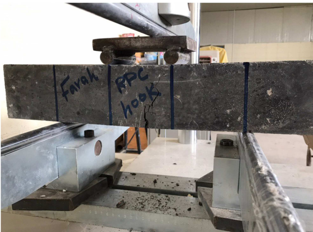
Figure 8. The failure mode of flexural strength test.
