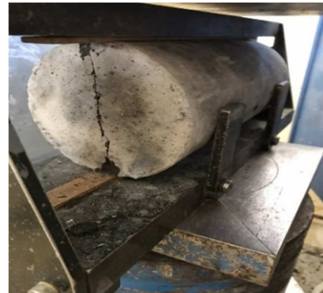
Figure 5. Effect of steel fiber type on splitting strength.
