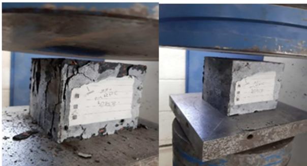
Figure 4. Mode of failure of compressive strength test.
