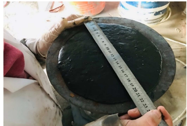
Figure 2. Flow Table test.
